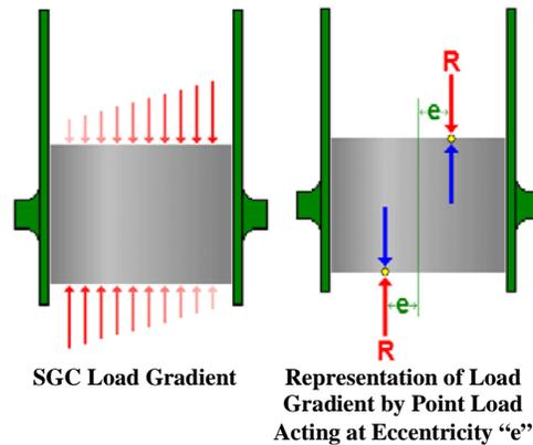
**Figure 12. Eccentric-Point-Load Concept Used by the RAM to Simulate Gyrotory Load**
