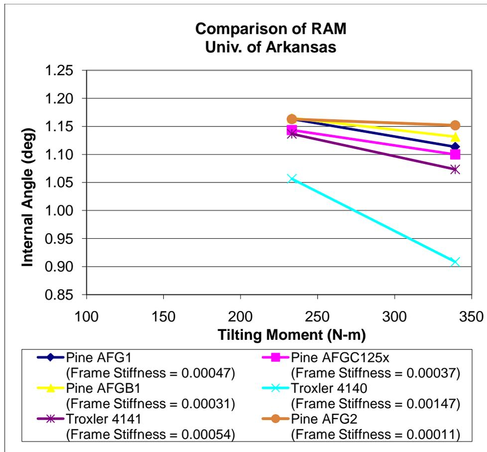
**Figure 17. Comparison of SGC frame stiffness using the Rapid Angle Measurement Device (RAM).**
