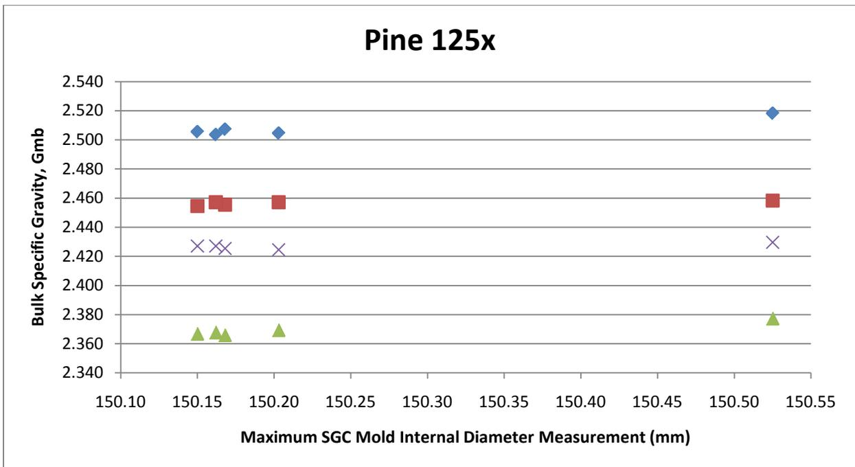
**Figure 4. Relationship Between Specimen Density and SGC Mold Diameter, Pine 125x**
