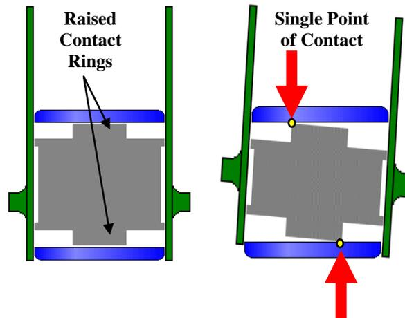
**Figure 14. RAM Simulation of Single Eccentric Point Load**
