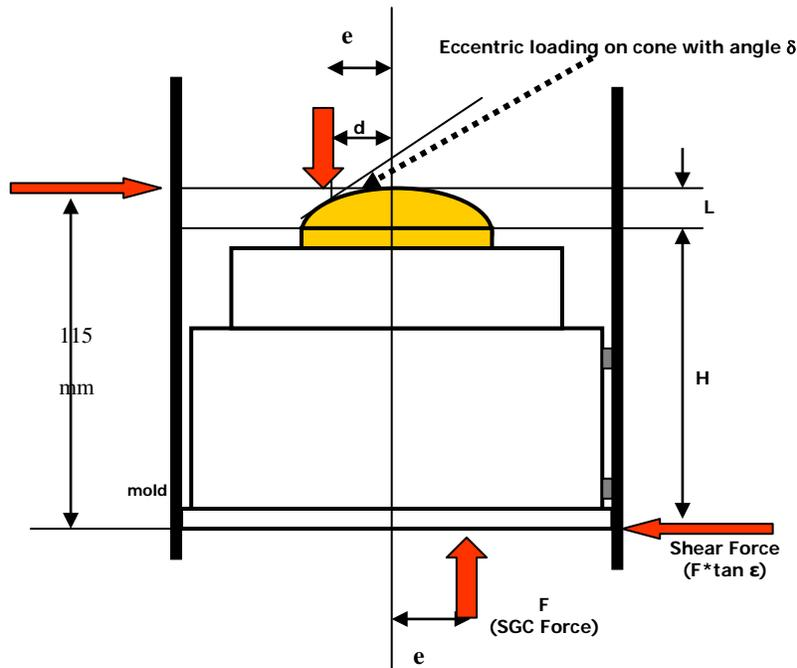
**Figure 16. Operational schematic of the Hot mix Simulator (HMS)**
