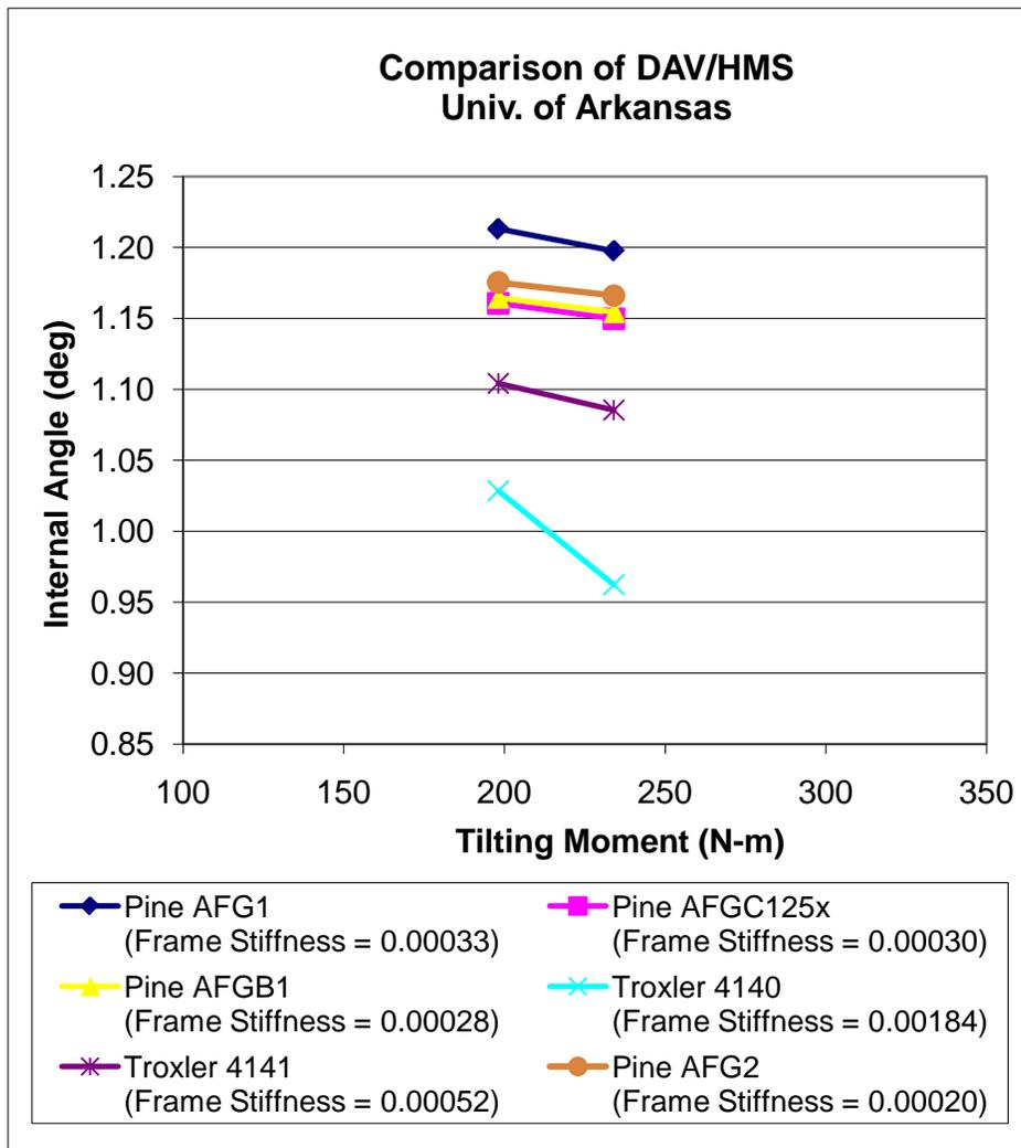
Figure 18. Comparison of SGC frame stiffness using the Hot mix Simulator (HMS).
