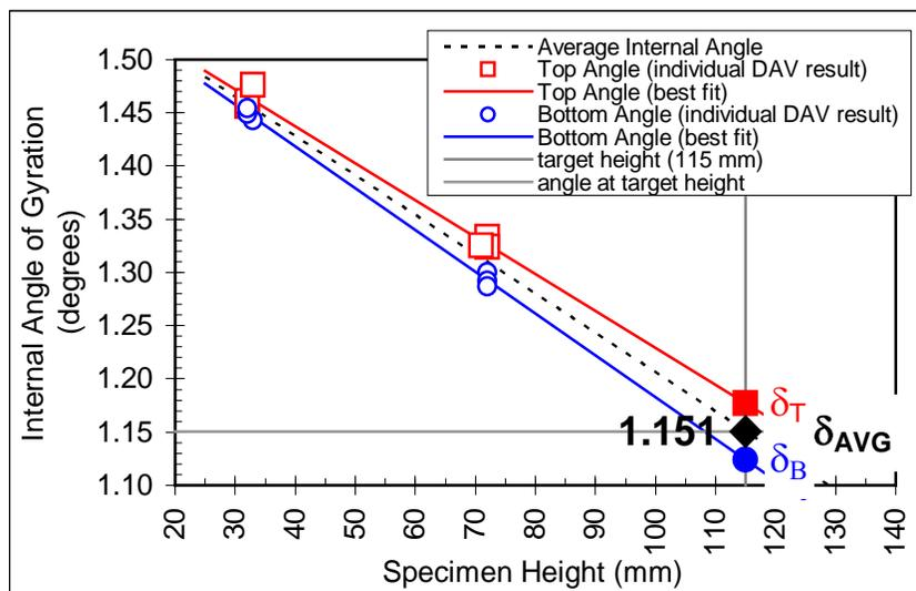
**Figure 9. Extrapolation Method for Determining Dynamic Internal Angle**
