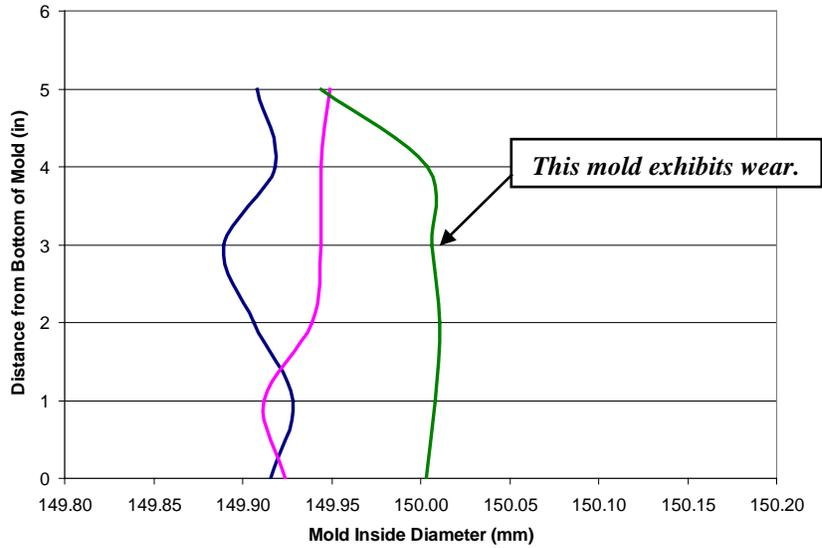
**Figure 1. Example of SGC Mold Diameter Measurement**
