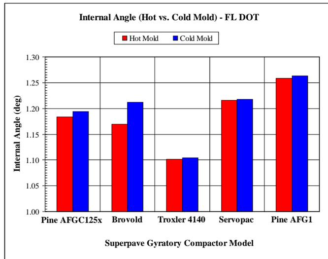
**Figure 19. Comparison of Internal Angle Values using Hot and Room-Temperature SGC Molds. (Data courtesy of Florida Department. of Transportation)**
